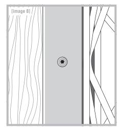
Now, place the element (for example wood) between the U-rails and affix it by using the enclosed clamp plate screws [image 5].
