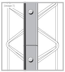
When the U-rails collide, the distance of 20 cm needs to be maintained.
