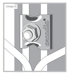
Fasten the U-rails above each crossing point of the column (every 20 cm) on the intended rectangular punchings by using a roundhead screw, locking nut and universal fixing clips.
