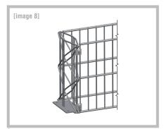
Screw the double rod gratings to the columns. The double rod gratings must be flush with the ground. Mounting is realized using universal clips [image 3] evenly distributed at the top and bottom (tighten hand-tight).
